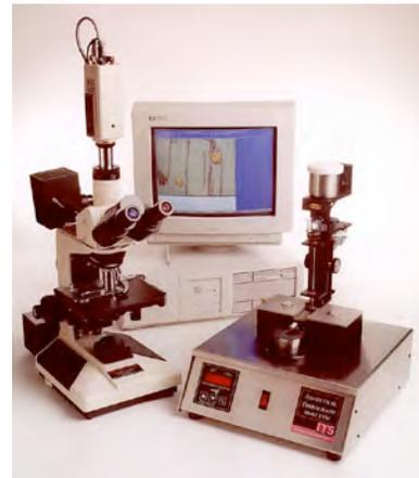
*Figure 2, T2FM Ferrography Laboratory*
